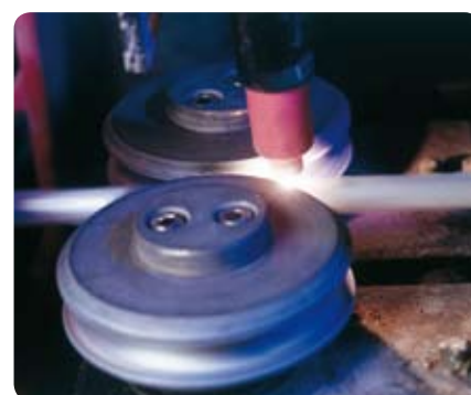
Fig 10. Laser welding Courtesy of Hewing
