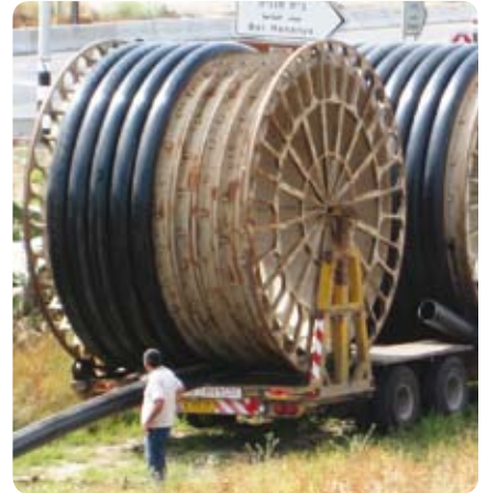
Fig. 25 Coil with big PE-Xa pipe Courtesy of Golan
